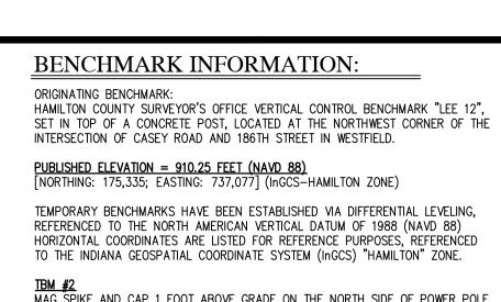
MAG SPIKE AND CAP 1 FOOT ABOVE GRADE ON THE NORTH SIDE OF POWER POLE "PSI 075 273", LOCATED ALONG THE NORTH SIDE OF WEST 193RD STREET APPROXIMATELY 490 FEET WEST OF THE INTERSECTION WITH CASEY ROAD. ELEVATION = 921.05 (NAVD88) [NORTHING: 179,278; EASTING: 736,590] (InGCS-HAMILTON ZONE)
